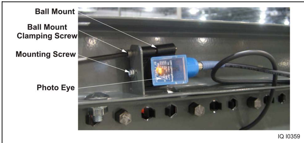
Figure 5 - 82 Photo Eye Mounting
