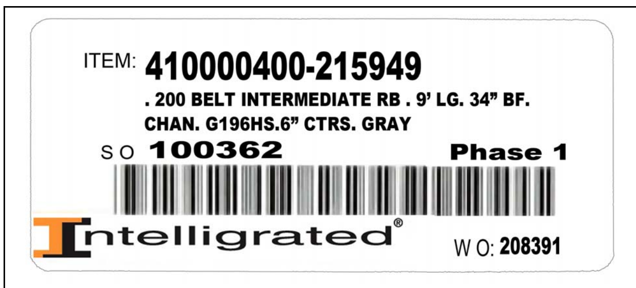
Figure 9 - 1 Example of Conveyor Label
