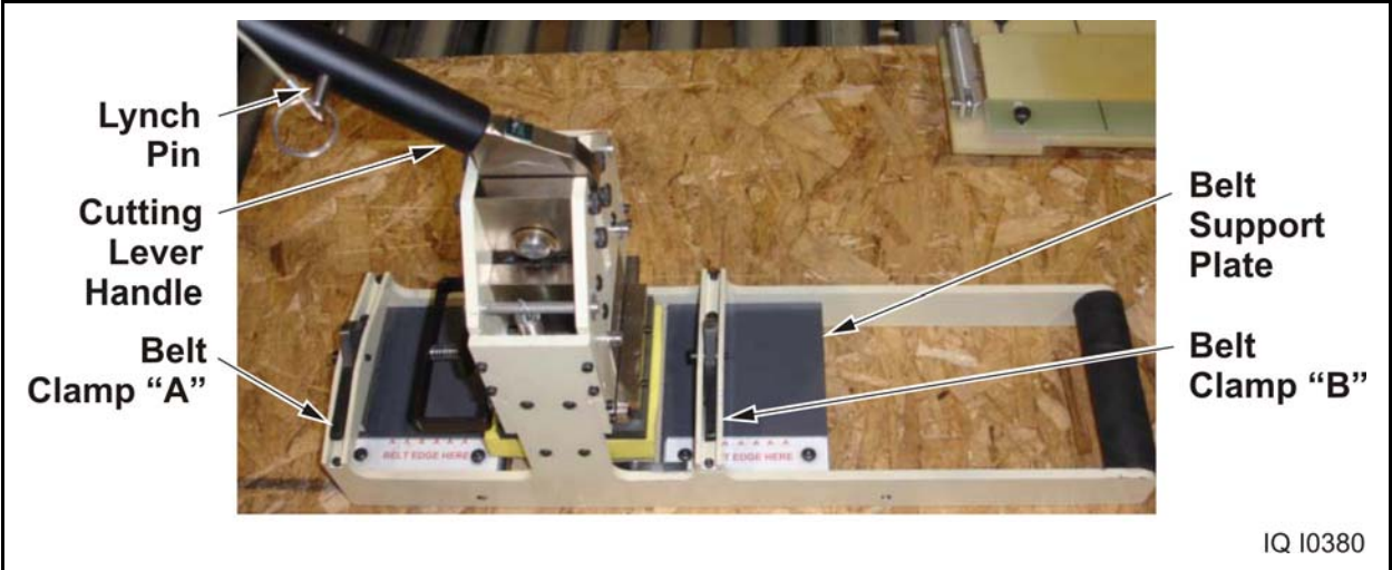
Figure 5 - 17 Preparing the Belt Cutter for First Cut
