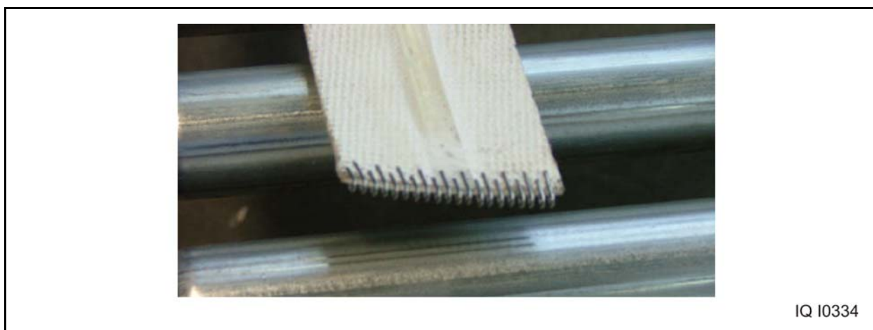
Figure 6 - 34 Proper Lacing Penetration
