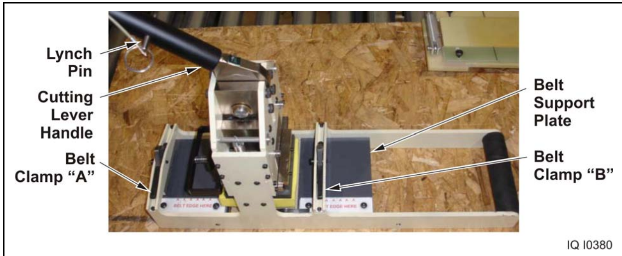
Figure 6 - 4 Preparing the Belt Cutter for First Cut
