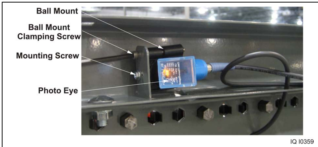
Figure 6 - 4 Photo Eye Mounting
