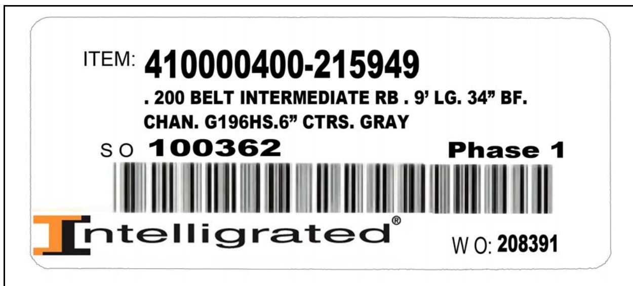
Figure 9 - 1 Example of Conveyor Label
