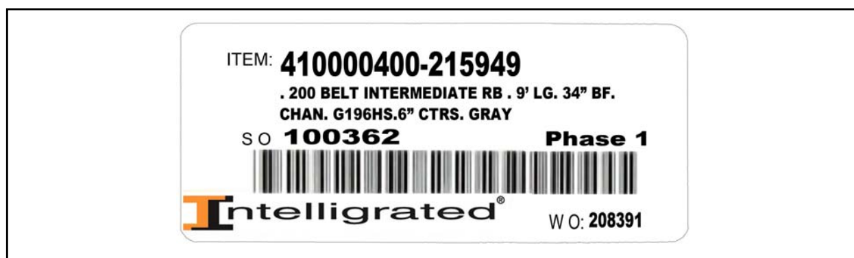
Figure 7 - 1 Example of Conveyor Label
