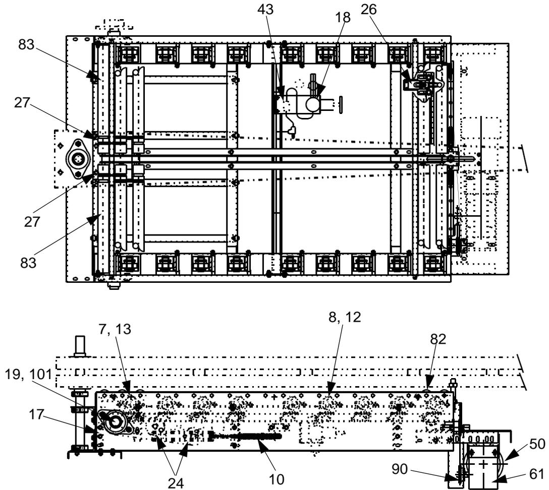
Figure I - 2 Powered Roller Diverge Unit
