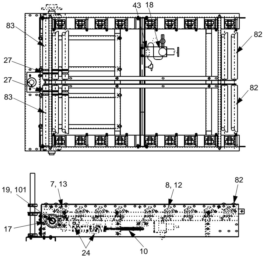
Figure I - 1 Powered Roller Merge Drive Unit
