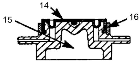
Figure I - 13 Diaphragm Actuator Components
