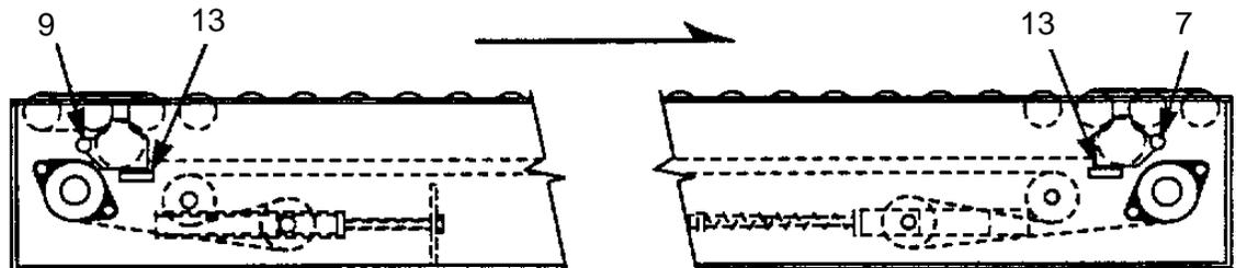
For DR Section Clutch (13) Only - Select RH/LH assembly that is opposite the mounting side
