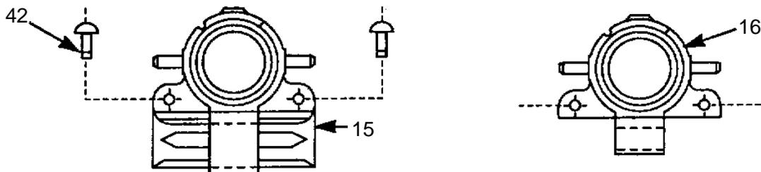
Figure I - 11 Intermediate Diaphragm Actuator (Left View)
