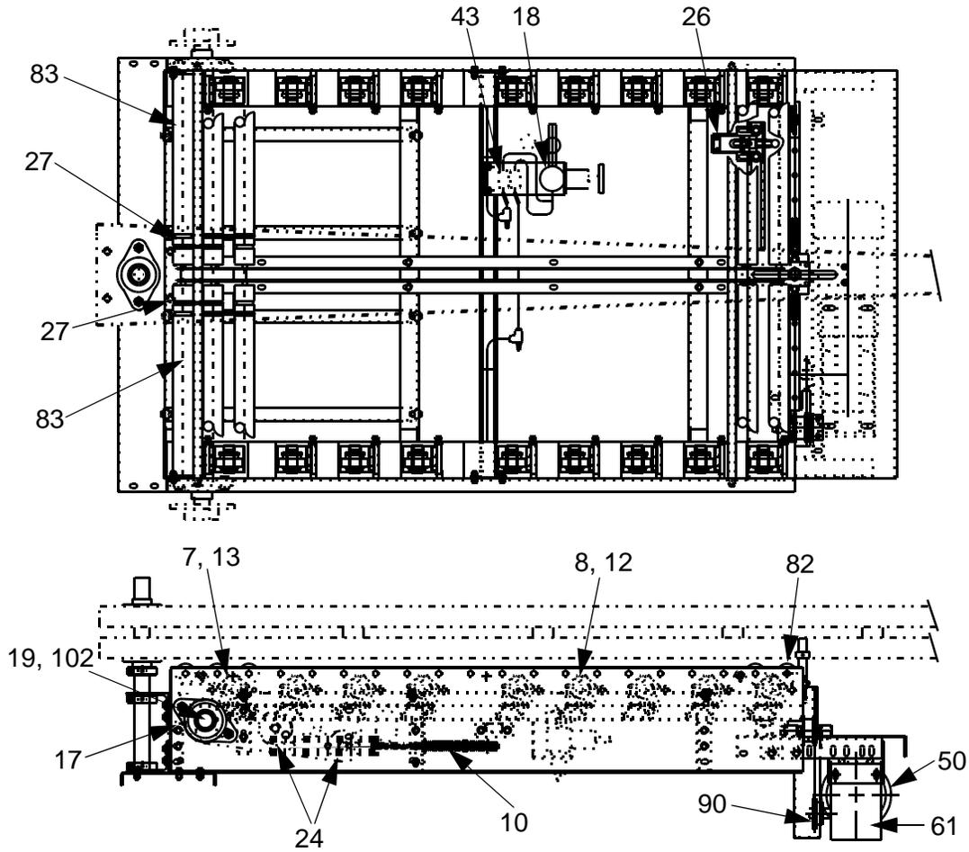
Figure I - 3 Powered Roller Crossover (PRC) Drive Unit
