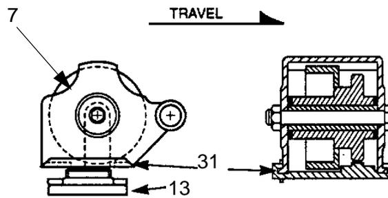
Figure I - 10 DR Section Clutch Components
