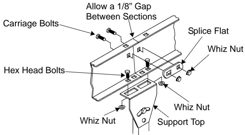
Figure G - 1 Standard Floor Support Assembly
