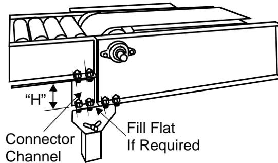
Figure G - 4 Connector Channel
