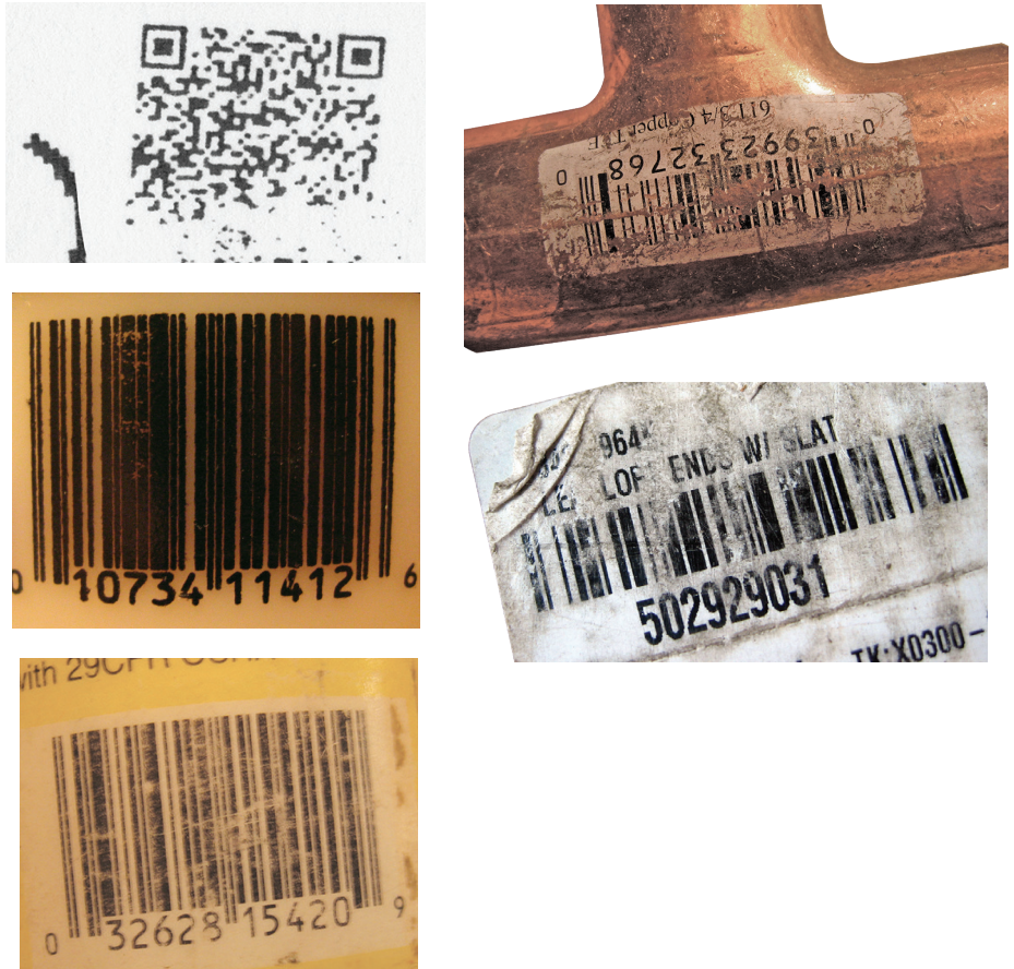
FIGURE 1. DAMAGED OR DISTORTED BARCODES
