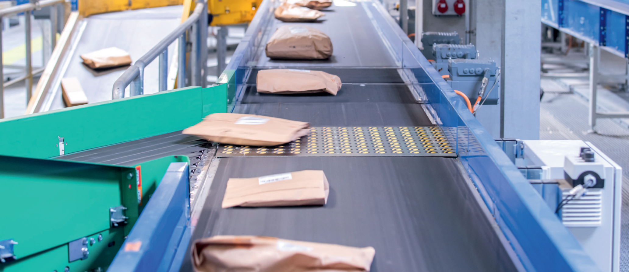
Easy maintenance access due to external drive components
