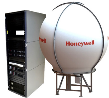
MEOLUT with mesh antenna
