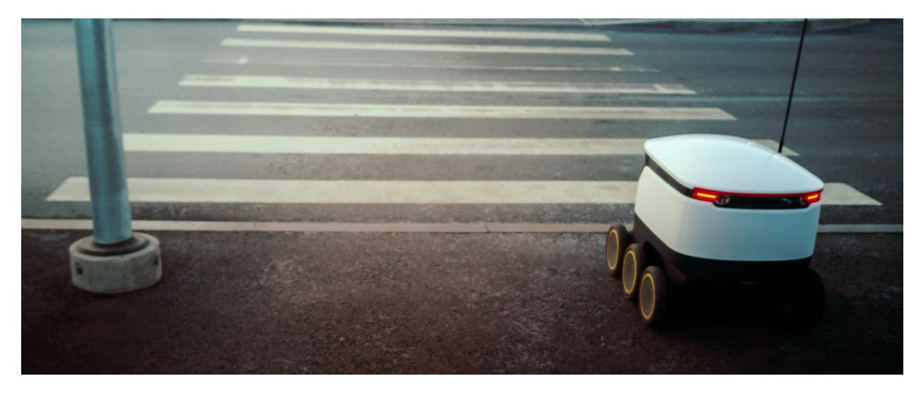
**Starship Technologies** uses rolling robots. Consumers receive their packages via a robot about the size of a cooler – no delivery person is involved!<sup>13</sup> The service is especially valuable for residential deliveries that required consumers to wait at home or visit a locker. This way, shoppers can get packages delivered when and where they want.
