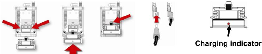
1. Align the Charging Adapter with the back of the RAELink3 Mesh (two guides match indents on the back of the Charging Adapter).
