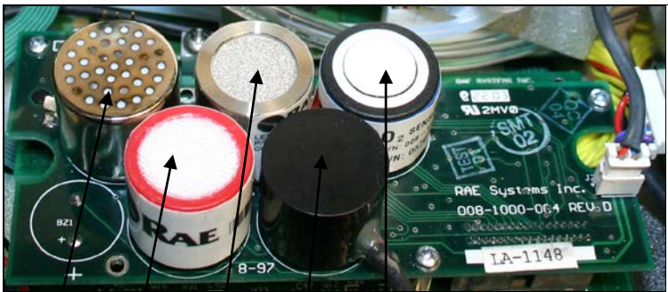
Figure 6-2 Gas Plate of AreaRAE
