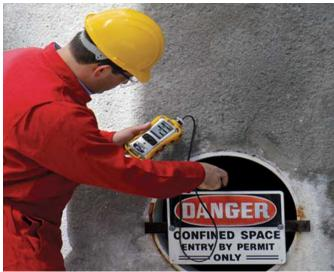
Most facilities utilize a combination of fixed-head gas detectors for area monitoring and portable gas detectors for personal protection.
